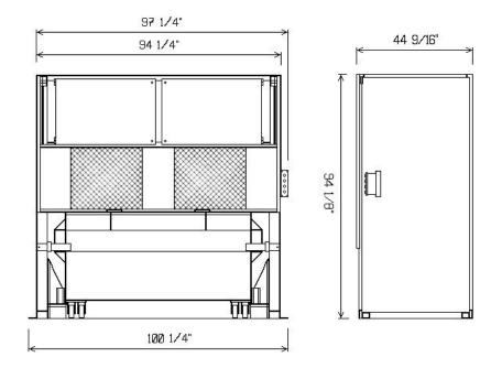
With a footprint barely  $4' \times 8'$ , the S-V2 fits where others won't. The S-V3 (with 3-yard container) is just 16" deeper at 62 3/4". Side-eject, right or left, available with slightly different dimensions.
